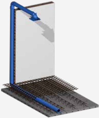
WIDE SLAB FLOOR
