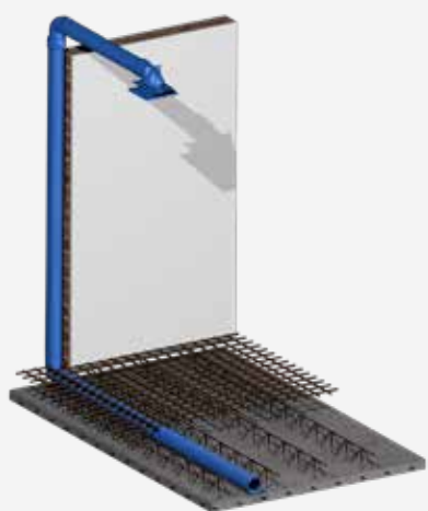
WIDE SLAB FLOOR
